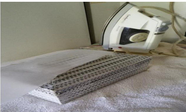
Figure 110. Sadeli box covered with veneering tape and with a sheet of bake paper, ready for the heat of the iron. Author's photo.
